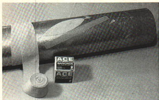
Left: The propeller blade twist is achieved by drying the wet blade on a section of 5-in. stovepipe (see text for more details). A 2-in. Ace bandage holds the blade in place. Right: Use this balsa prop jig to assemble sizes from 12- to 14-in. in diameter and from 22- to 28-in. in pitch.
